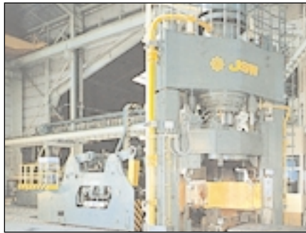
Forging Pump Pump Used: K3VG280DT
